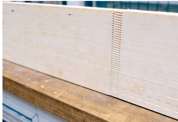
The quality of the finger joints plays a central role at Theurl. Since using LEUCO fingers with Solid 34 cutting material and topcoat coating, Theurl has recorded almost constant finger jointing quality over the entire edge life of around 600,000 cycles.
