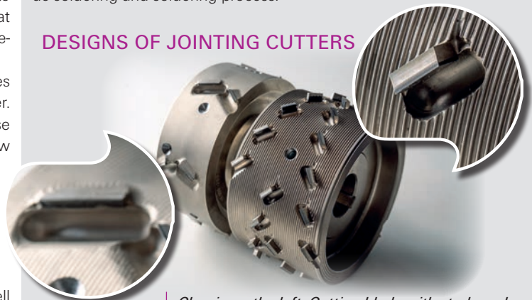
Classic on the left: Cutting blade with studs and balancing bores. On the right, the DIAMAX and DIAREX airFace principle: Cutting blade directly in the base body, balanced using balancing screws
