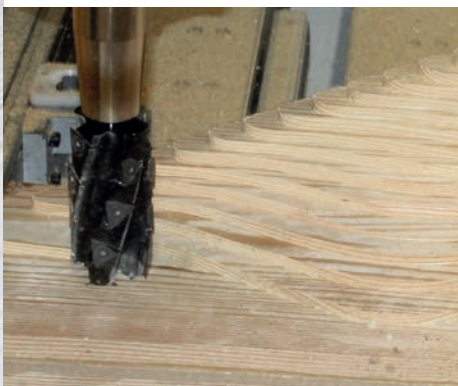
The surfaces and edges in ash produced by the LEUCO t3-System shank-type cutter are smooth and chip-free.
