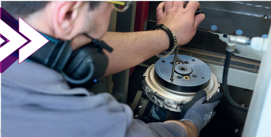
Minimal machine down-time, maximum cutting edge utilization: a sharp cutting edge area is set with a small turn
