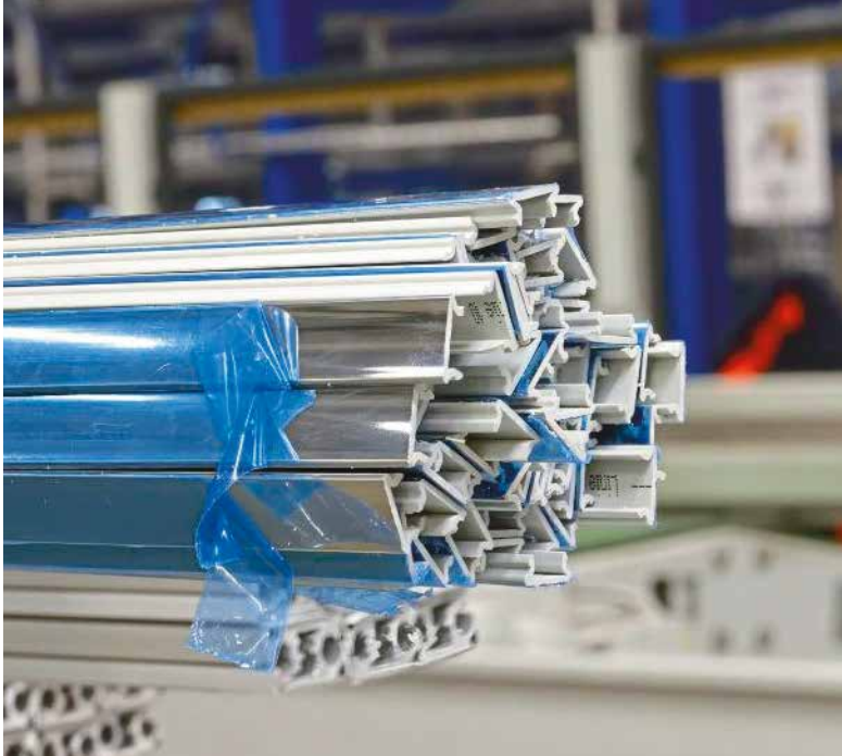
This bundle of chrome-plated plastic strips was cut in its entirety by the saw. Regardless of the random location of a profile, the quality is always right.
