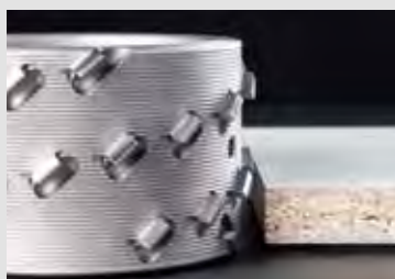
Standard DIAREX airFace Z3+3 cutter - engagement of the cutting edges in the panel. Adjustment of the cutter height to the 19-mm panel must be precise so that the overcut area does not reach the upper melamine layer.
