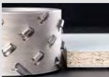
Fibonacci DIAREX airFace Z3+3 cutter: The Fibonacci arrangement ensures that there is no overcut area. One cutting edge always mills the upper edge of the material exactly without chipping - this is called freedom from height adjustment.
