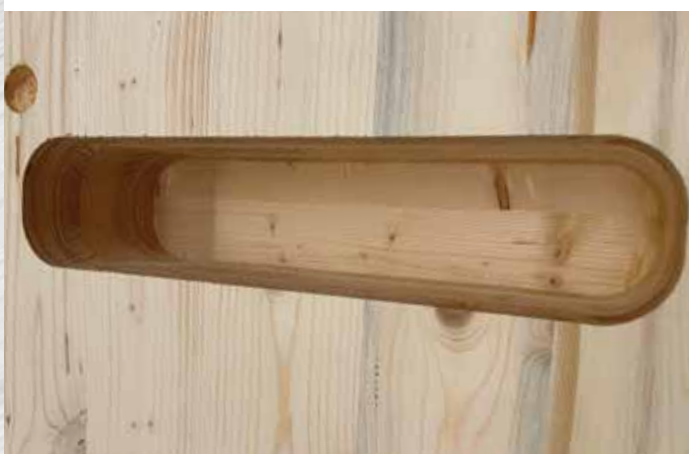
High chip volume quickly disposed of and a clean edge: spiral plunge into the material with the t3-System multi-block cutter at a feed rate of 10 meters and 8,500 rpm.
