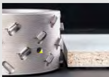
Fibonacci DIAREX airFace Z3+3 cutter: The Fibonacci arrangement ensures that there is no overcut area. One cutting edge always mills the upper edge of the material exactly without chipping - this is called freedom from height adjustment.
