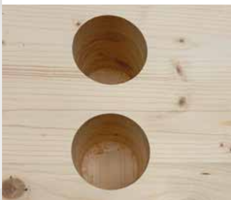
High chip volume quickly disposed of and a clean edge: spiral plunge into the material with the t3-System multi-block cutter at a feed rate of 10 meters and 8,500 rpm.
